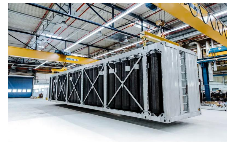
HexagonPurus mobile hydrogen distribution systems
