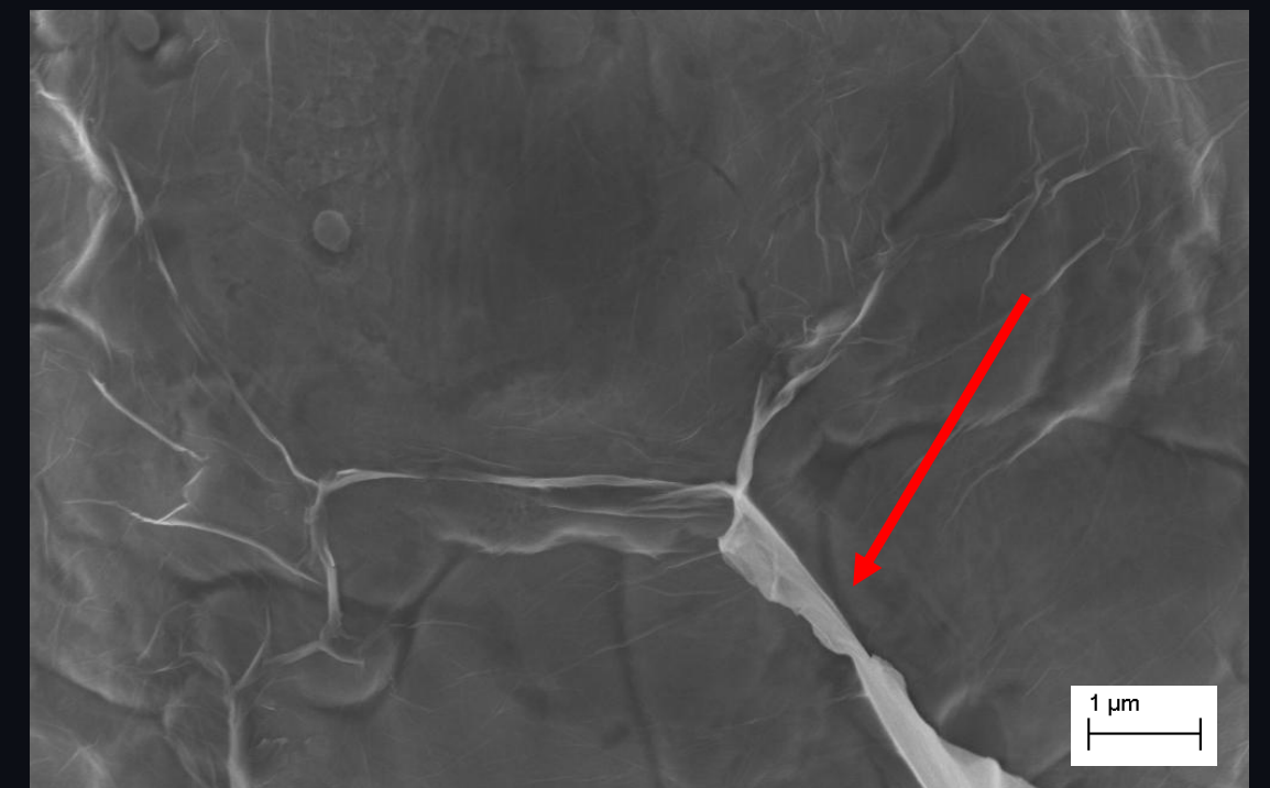
316L powder coated with graphene oxide
